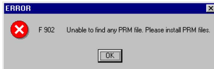
Figure 4-1. Fatal Error: No Parameter File Installed
